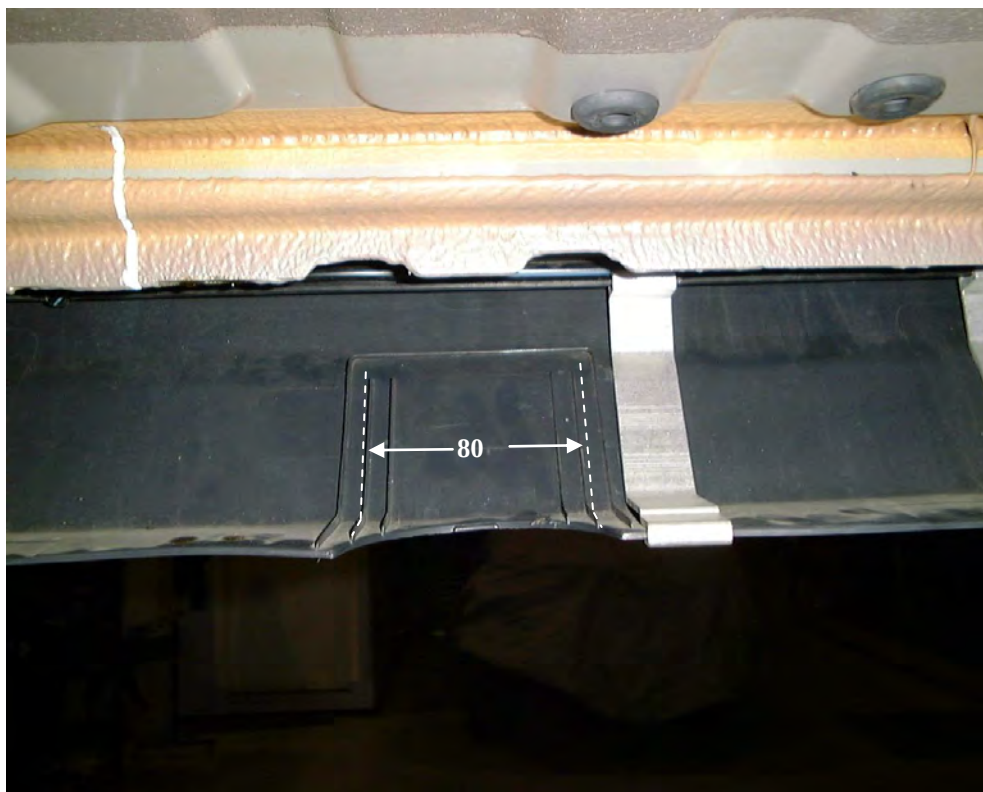
Bumper cut diagram 1, use fins on bumper as a guide.
