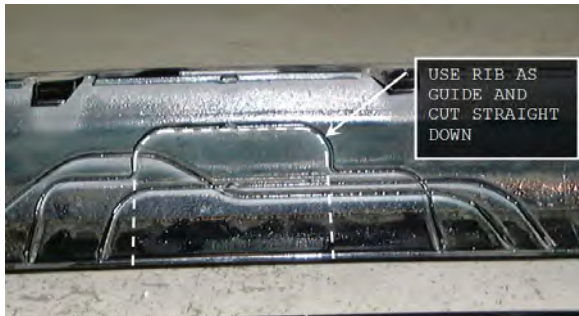
Figure 1 – Bumper cut out illustration for Sedan.
