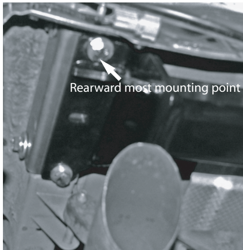
Figure 6: Attach LHS to mounting brackets.
