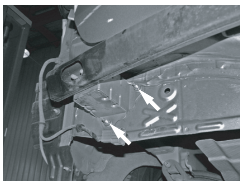
Figure 3: Remove rear impact beam.
