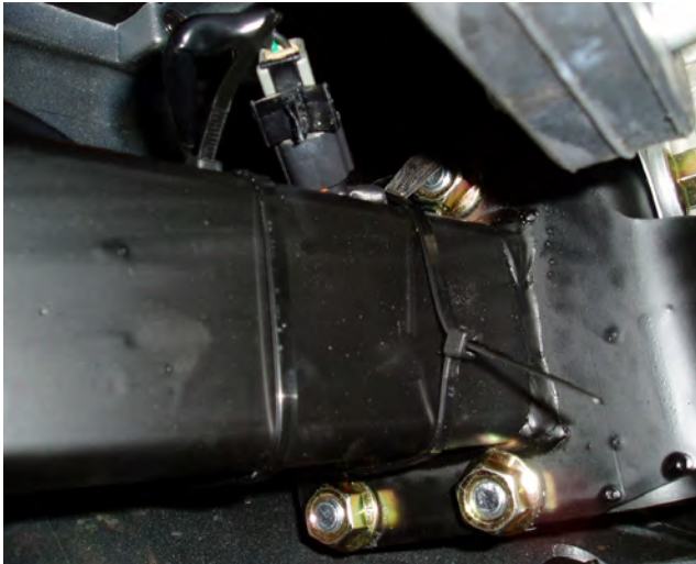
Fig 5: Shows the heat shields to be trimmed.
